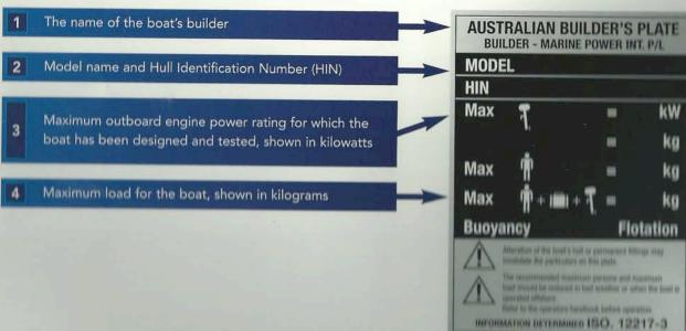
Maximum outboard engine weight for which the boat has been designed and tested, shown in kilograms
